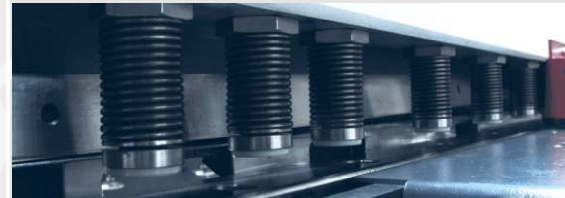
Hold Down Pads
