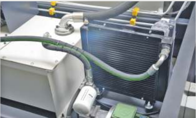
Hydraulic Oil Cooling System
